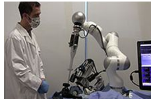
University of Maryland surgeon supervising the Smart Tissue Autonomous Robot (STAR). Source: University of Maryland
